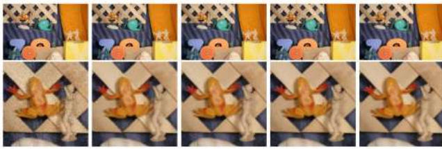
Figure 14: Visual comparison with simulated noisy CFAs. From left to right: image by local demosaicking, image by temporal demosaicking plus VBM3D, proposed demosaicking, proposed CFA denoising plus local demosaicking and complete chain.
